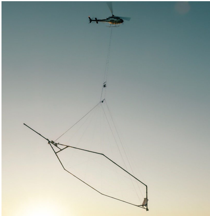
Figure 13. Helicopter collecting AEM data in Middle Republican NRD.
