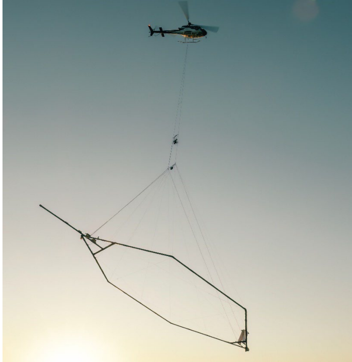
Figure 14. Helicopter collecting AEM data in Middle Republican NRD.
